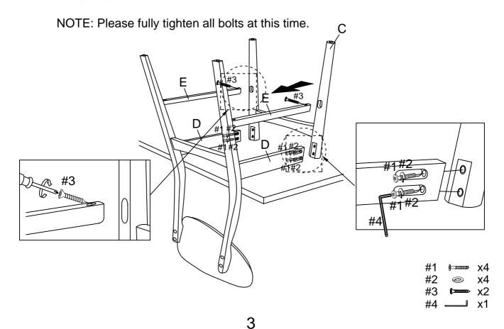
Step 3 . Attach seat (part B) to assembled unit (parts A, C, D & E) using screws (part #3) and phillips head screwdriver.
