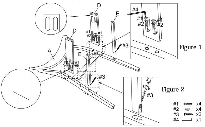
Step 2 . Attach front leg (part C) to side rails (part D) and strechers (part E) using bolts (part #1), spring washers (part #2), screws (part #3), allen wrench (part #4) and phillips head screwdriver.
